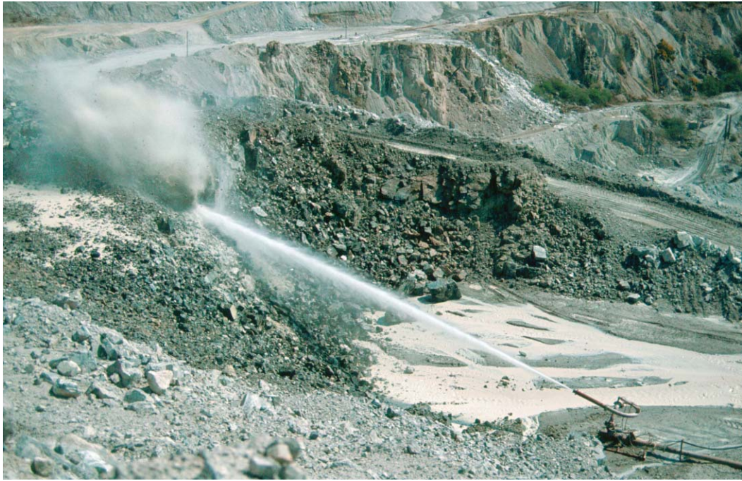
Figure 1-5. Hydraulic mining of china clay from the strongly kaolinised St Austell granite. Waste materials from this important industry are quartz-rich sands. They are very stable and usually have ideal natural grading for concrete aggregates. China clay waste is the most widely used concrete aggregate in the region.
