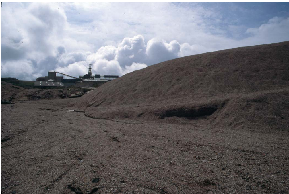
Figure 1-1. Processing waste from granite-hosted tin mineralisation at the former Geevor Mine, near St Just - a stable Group 1-6 aggregate.
